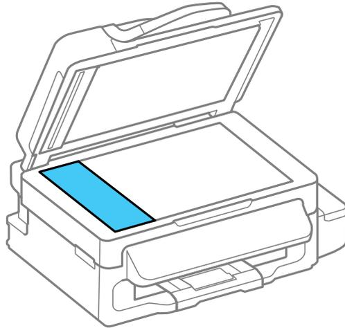
6. Open the ADF cover and use a soft, dry, lint-free cloth (microfiber is recommended) to clean the rollers and the interior of the ADF.
