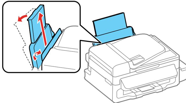
2. Pull out the output tray and open the paper stopper on the end.
