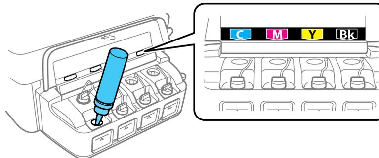
5. Snap off the tip of the bottle cap, but do not dispose of it so you can use it to seal the bottle cap later, if necessary. Then remove the bottle cap and carefully remove the protective seal (avoid touching the ink underneath the seal). Close the bottle cap tightly.
