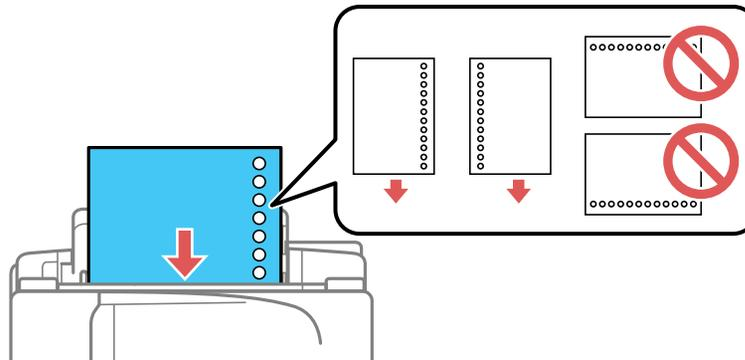
6. Slide the edge guide against the paper, but not too tightly. Then, flip the feeder guard back.
