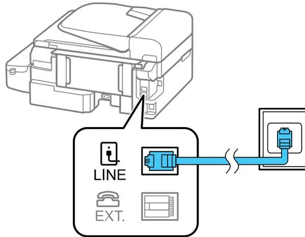
**Note:** If you have a DSL or ISDN connection, you must connect the appropriate DSL filter, or ISDN terminal adapter or router to the wall jack to be able to use the line for faxing or voice calls using your product. Contact your DSL or ISDN provider for the necessary equipment.
