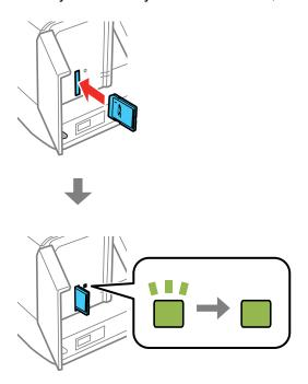
**Note:** Do not force the card all the way into the slot. Insert it only until it meets resistance.
