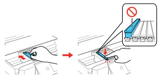
8. After you replace all the cartridges that need replacing, lower the scanner unit and select **Completed** on the LCD screen.
