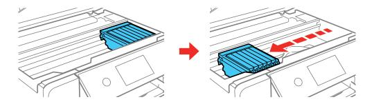
**Caution:** Do not move the print head by hand or use any kind of tool to remove a cartridge; otherwise, you may damage your product. Do not touch the flat white cable or the metal bar inside the product.
