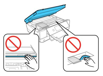
3. Push in the blue tab to unlock the ink cartridge you are replacing. Then lift the ink cartridge as shown to remove it.
