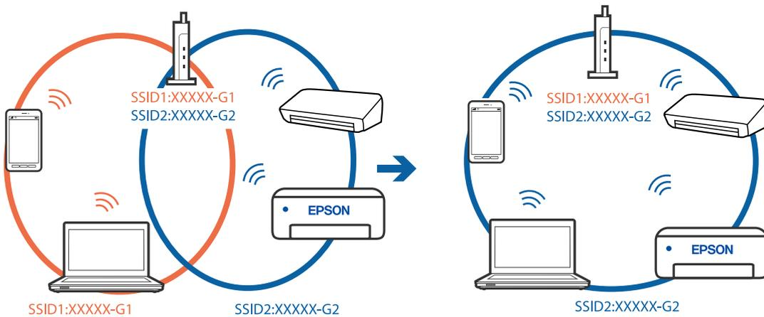
❑ Example of connecting to SSIDs with a different frequency range
