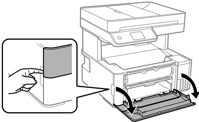
7. Lower the output switch lever.
