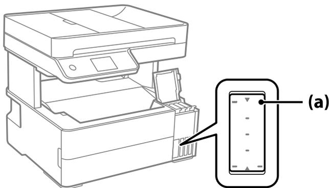
8. Align the top of the ink bottle with the filling port, and then insert it straight into the port to fill ink until it stops automatically at the upper line.
