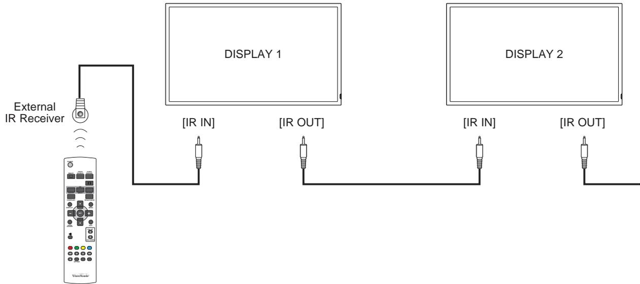
**NOTE:** This display's remote control sensor will stop working if the [IR IN] is connected.
