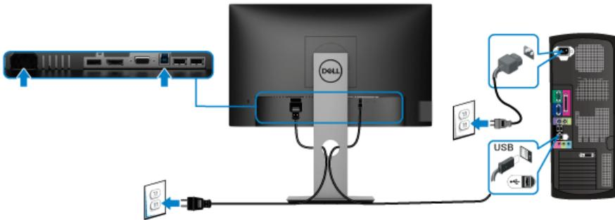
1. Connect the upstream USB 3.0 port (cable supplied) to an appropriate USB 3.0 port on your computer. (See [Bottom view](#) for details.)
