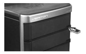
When the disk tray slides open, place the CD or DVD gently on the tray. Make sure that the label or title side of the disk is facing upward. When holding a disk, hold it by the edges to avoid leaving smudges or fingerprints.
