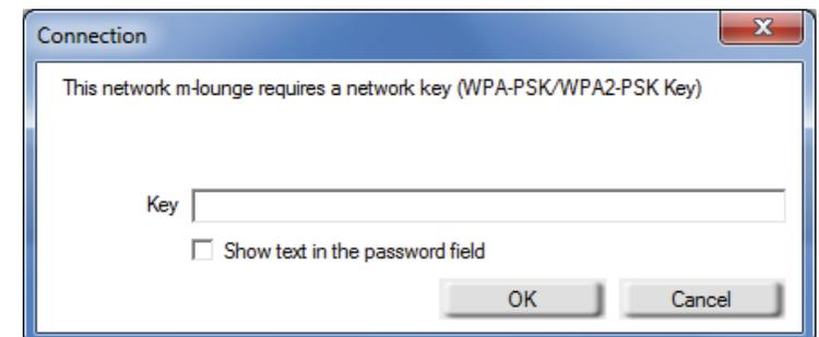
It is recommended to enable WPA/WPA2-Personal on your wireless router or access point before configuring your wireless adapter. Make sure you enter the passphrase exactly the same on all wireless devices.
