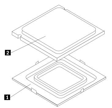
Step 9. Holding the sides of the microprocessor with your fingers, position the microprocessor so that the notches on the microprocessor are aligned with the tabs in the microprocessor socket.
