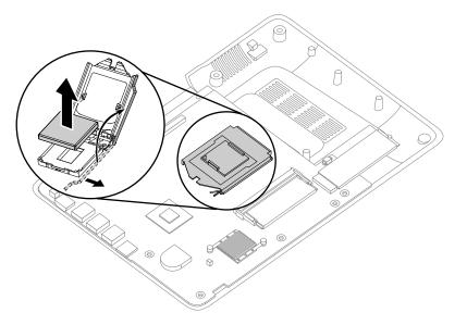
**Attention:** Do not touch the gold contacts on the bottom of the microprocessor. When handling the microprocessor, touch only the sides.
