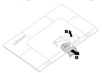
Step 6. Working around the edge in an anti-clockwise direction, use your fingers to prise up the rear cover. The rear cover is pinned into place, use short, sharp movements to prise it up.
