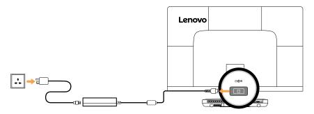
Step 3. Connect the new adapter as shown.
