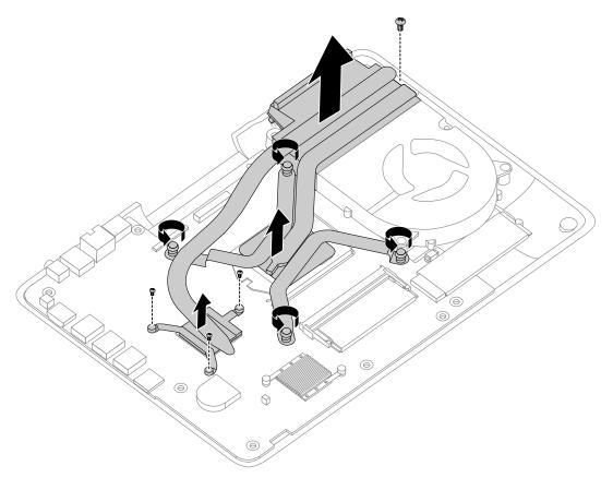
Attention: Place the heat-sink upside down on a flat surface to prevent thermal grease from contaminating other components.
