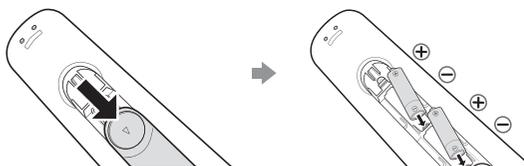
After you have installed the batteries, use a screwdriver to screw in the screw that holds the battery cover closed.
