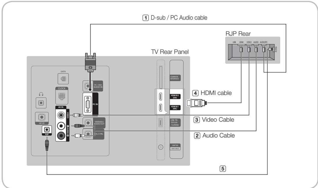
1. Connect the PC IN / PC/DVI AUDIO IN port of the TV to the PC/AUDIO port of the RJP.
