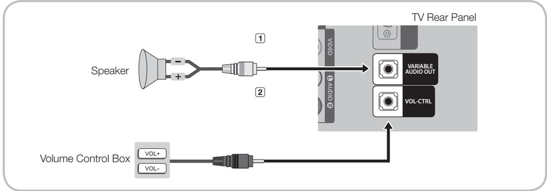
1. Connect the **VARIABLE AUDIO OUT** port of the TV to the Bathroom Wall Speakers of the hotel.
