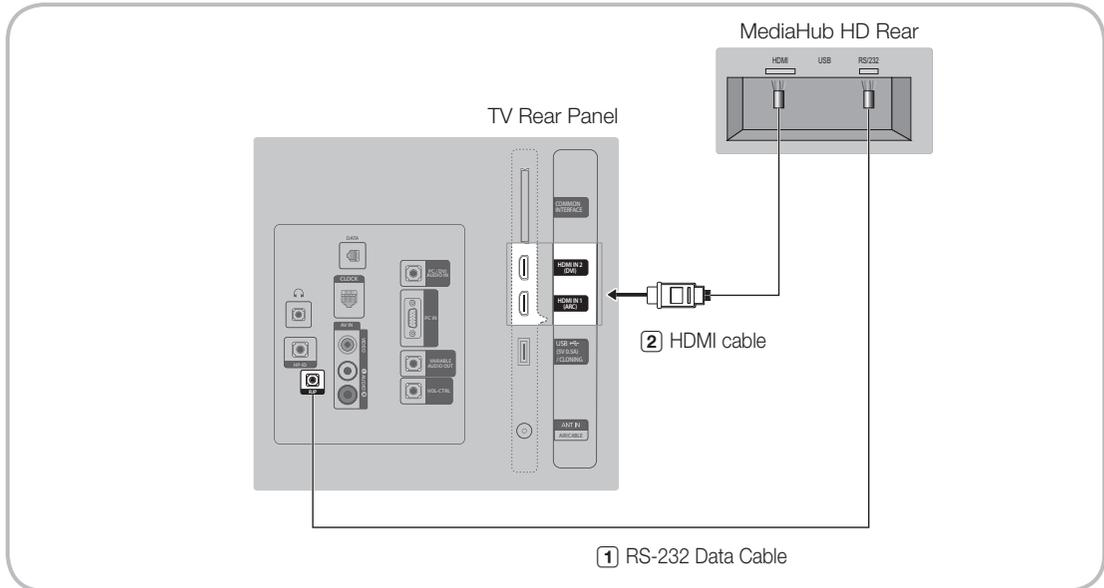
1. Connect the RJP port of the TV and the RS/232 port of the MediaHub HD.
