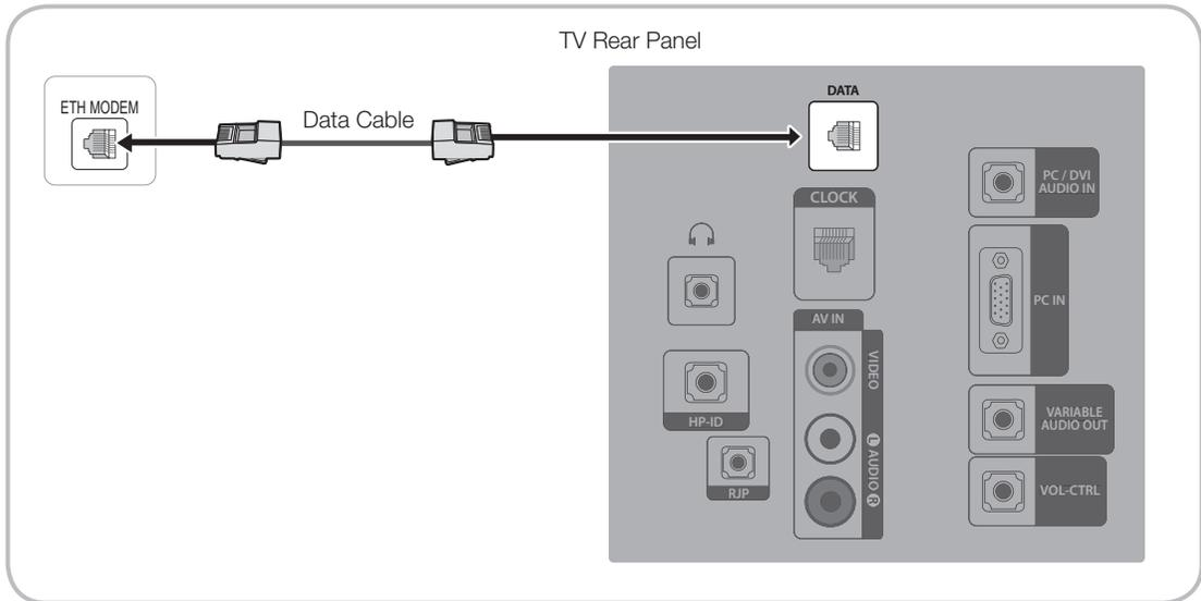
1. Connect the DATA jack of the TV to the [ETH MODEM] jack of the STB (SBB) with the Data cable.
