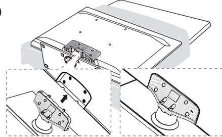
Place a soft cloth over a table to protect the TV, and then place the TV on the cloth screen side down.
