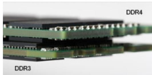
**Figure 2. Thickness difference**
