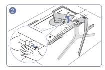
Push the key upward and hold. Turn the stand neck After turning the stand neck of the display of the display counterclockwise for 10°.
