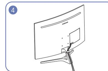
Connect the power supply and the data cable as shown in the figure.
