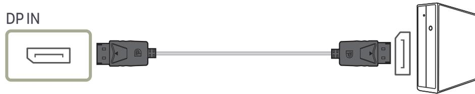
— A DP cable shorter under 1.5 m in length is recommended. Using a cable longer than 1.5 m can affect the picture quality.
