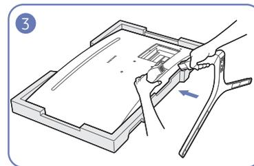
Place the protective Styrofoam (cushion) included in the package on the floor and place the product facing down on the Styrofoam, as shown in the image. If Styrofoam is unavailable, use a thick sitting mat. Hold the back of the monitor as shown in the figure. Push the assembled stand into the main body in the direction of the arrow as shown in the figure.
