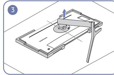
After turning the stand neck of the display counterclockwise for 10°, lift the stand neck to detach it from the device.
