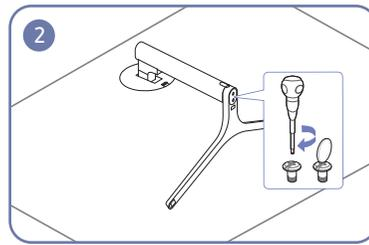
Check that the stand neck is firmly connected. Tightly fasten the connecting screw at the bottom of the stand base.
