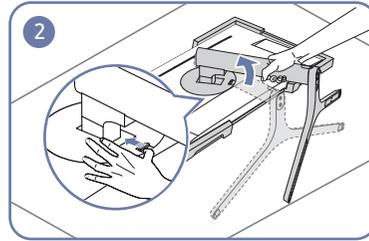
Push the key upward and hold. Turn the stand neck of the display counterclockwise for 10°.
