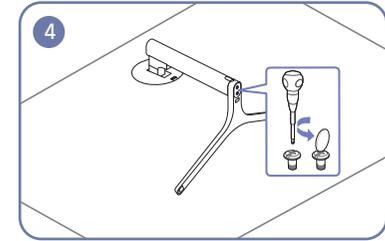
Turn the connecting screw at the bottom of the stand base to separate it.
