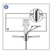
Insert and fix the cables in the slot.
