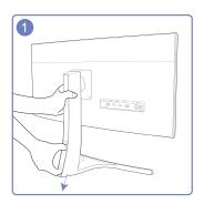
To remove the COVER-CABLE, hold and pull the COVER-CABLE with your thumb and index finger in the arrow direction while holding the stand with the other hand.
