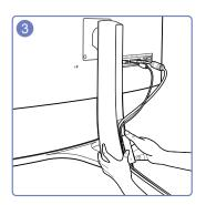
Hold the COVER-CABLE and fix the cables into the grooves on the STAND-REAR.
