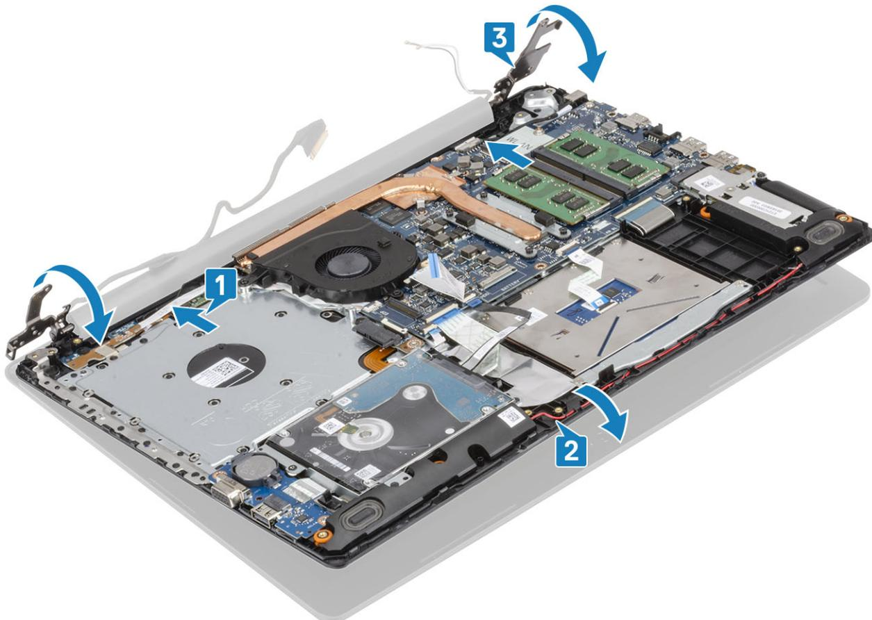
4. Replace the five (M2.5x5) screws that secure the left and right hinges to the system board, and palmrest and keyboard assembly [1].
