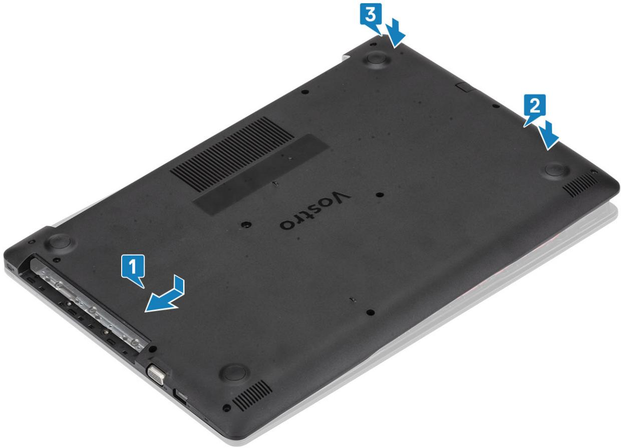
3. Tighten the three captive screws, and replace the single (M2x4) screw that secures the base cover to the palmrest and keyboard assembly [1, 2].
