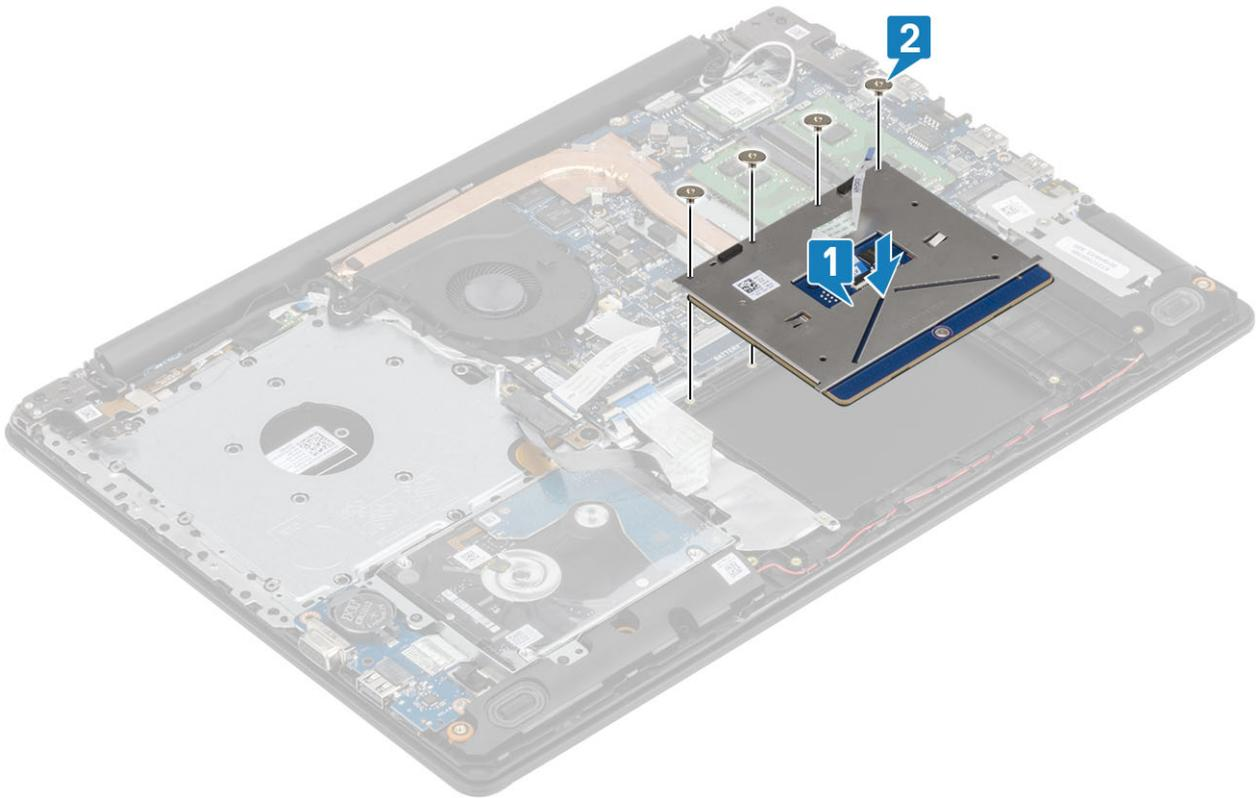
3. Place the touch pad bracket into the slot on the palmrest and keyboard assembly [1].
