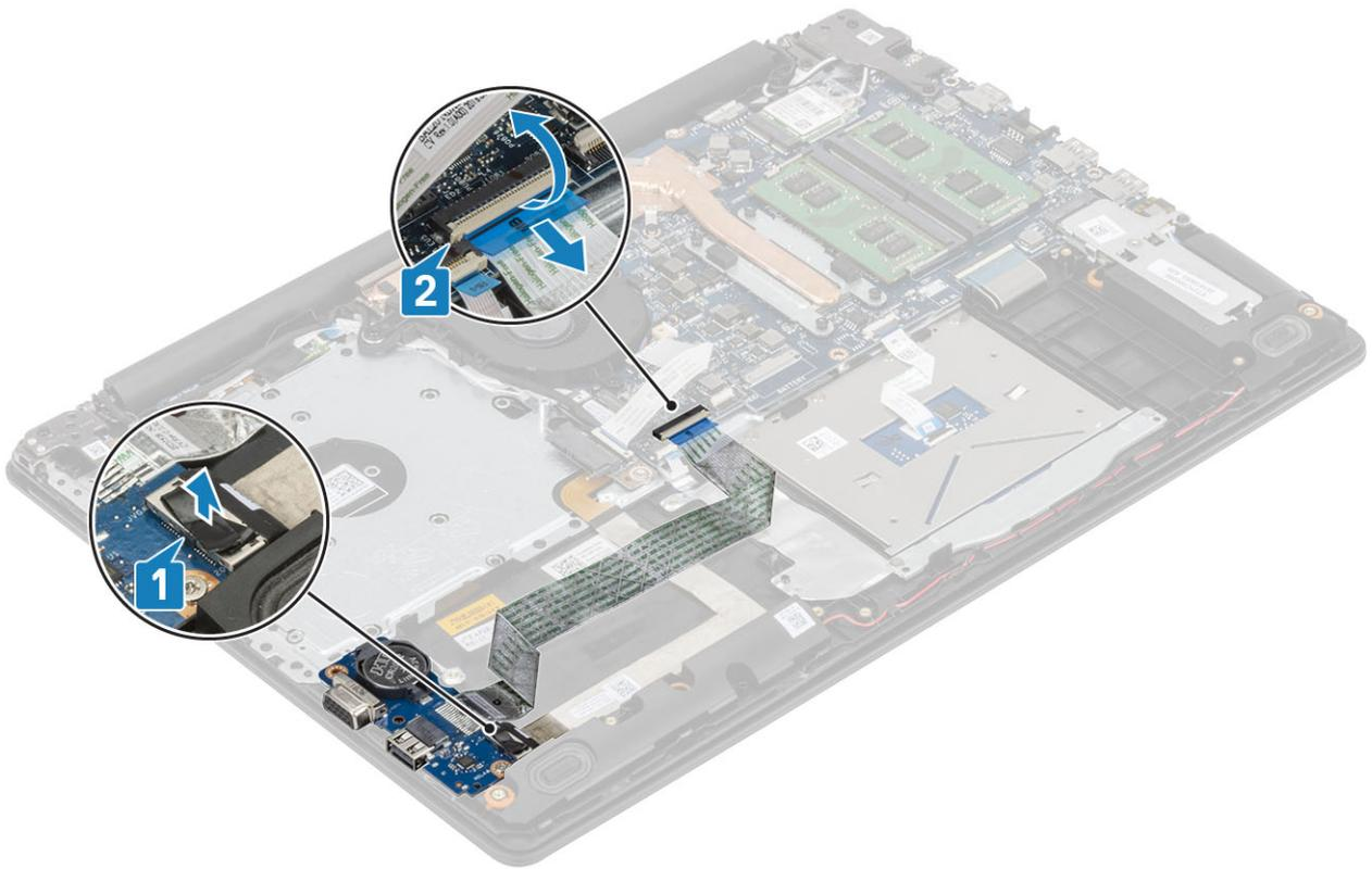
3. Remove the single (M2x4) screw that secures the I/O board to the palm rest and keyboard assembly [1].
