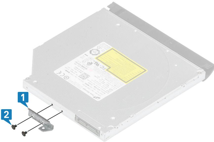
3. Insert the optical drive into the slot until it clicks into place [1].
