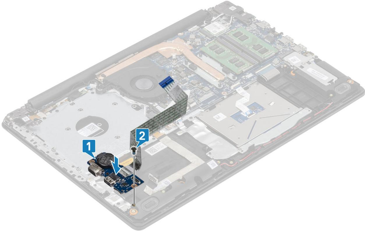
3. Connect the VGA cable to the I/O board [1].
