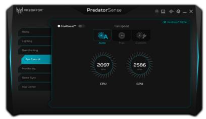
Activate **CoolBoost™** to increase fan speed beyond the normal maximum, enhancing cooling power when the system is under heavy use.
