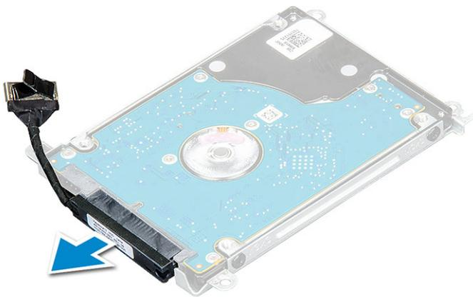
5 Then, remove the M3xL3 screws to detach the bracket from the HDD.
