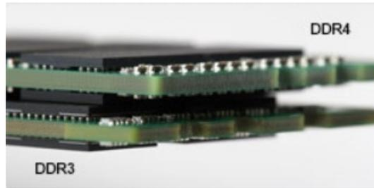
**Figure 2. Thickness difference**
