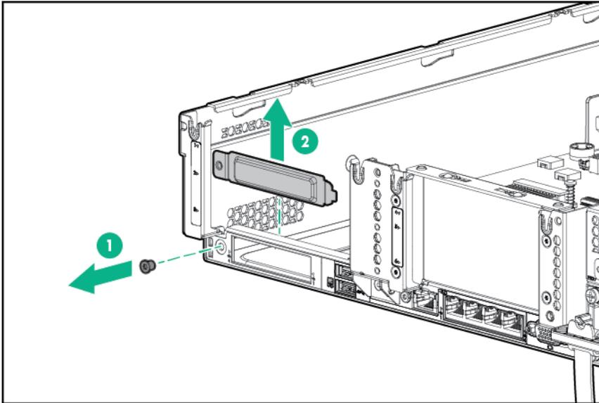
7. Install the FlexibleLOM adapter:
