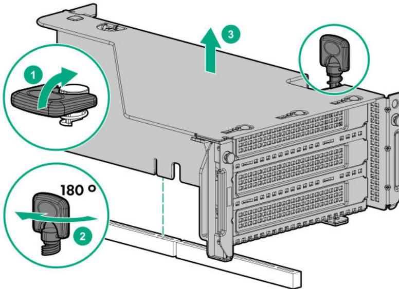
6. Remove the rear wall blank.
