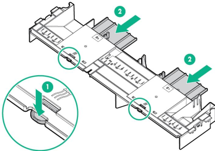
8. Install the appropriate retention clip onto the air baffle.
