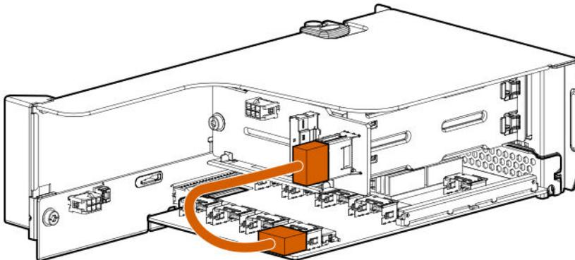
Rear 2SFF drive option in the secondary slot to a SAS Expander in primary slot
