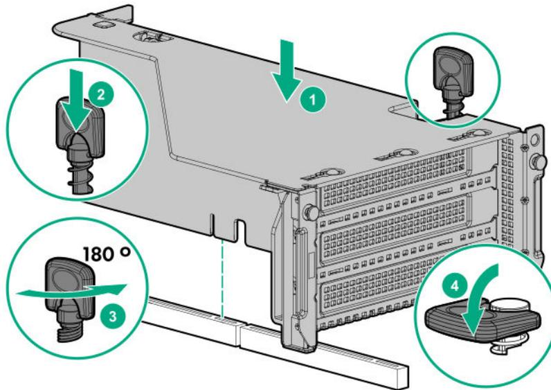
17. Slide the retention clips to the locked position.
