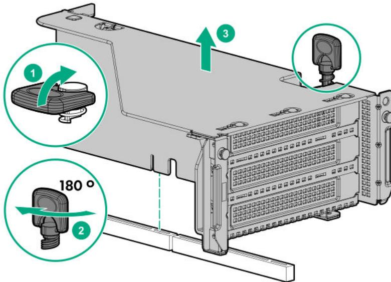
Remove the secondary wall blank.
