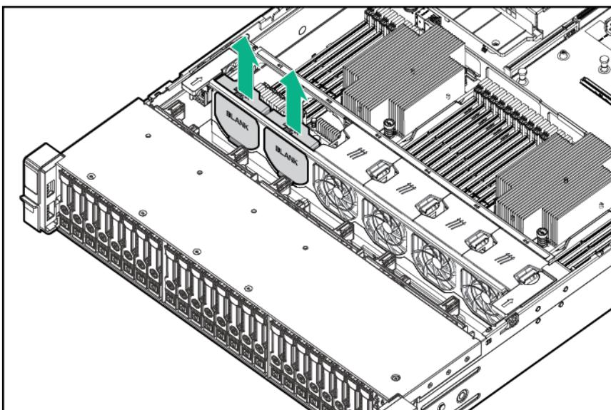
4. **Remove the air baffle.**
