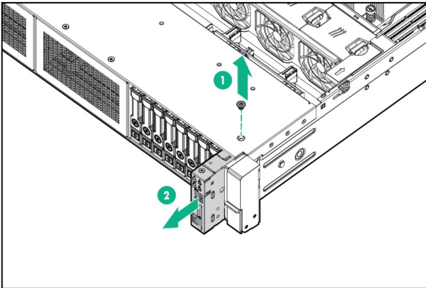
9. Route the cable through the opening in the front of the server, and then install the SID power switch module. Secure the module using the existing screw.
