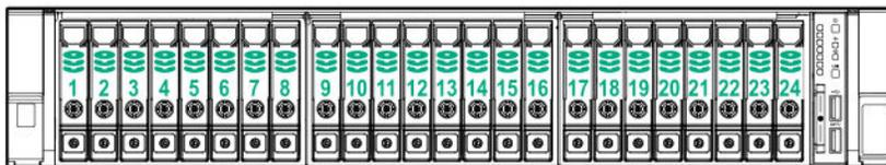
When any stacked 2SFF drive cage is connected to the SAS expander, the drive numbering skips the second number to allow **uFF drive bay numbering** on page 31. For example, when a rear 2SFF drive cage is connected to SAS expander port 9, then the drive numbers are 25 and 27.
