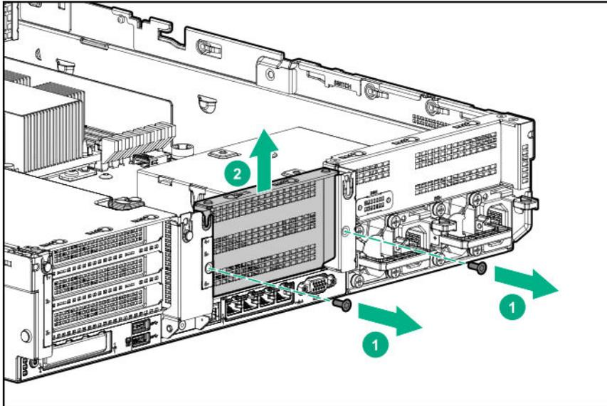
12. Remove the PCIe blank.
