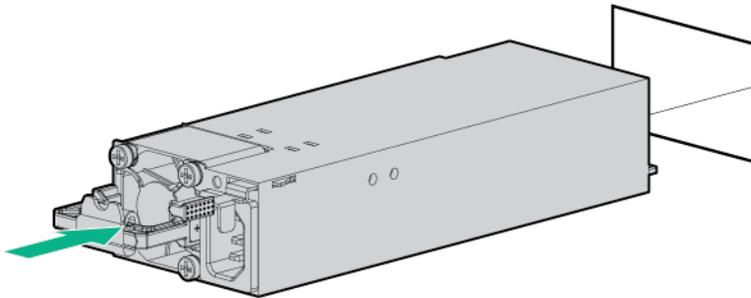
4. Connect the power cord to the power supply.
