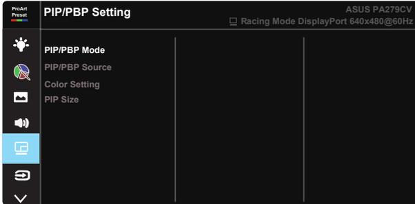
By activating this function, this monitor displays two pictures, three pictures or four pictures for any video source.
