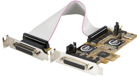
The PEX8S950LP 8 Port PCI Express Low Profile Serial Adapter Card with dongle cables included offers 8 RS 232 Serial connections via a single PCI Express slot, with data rates up to 921Kbps. Perfect for use with a broad variety of serial peripherals including printers, scanners, industrial controls and more.
