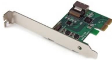
The PEXSAT34SFF PCI Express SATA Controller Card enables 4 AHCI SATA III connections to be added to a computer, through a single internal Mini-SAS (SFF-8087) port, connected using a PCI Express slot.
