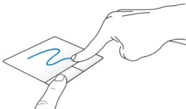
Select an item then press and hold the left button. Using your other finger, slide down the touchpad to drag and drop the item to a new location.
