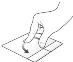
With one finger steady on the touchpad, rotate another finger clockwise or counterclockwise.
