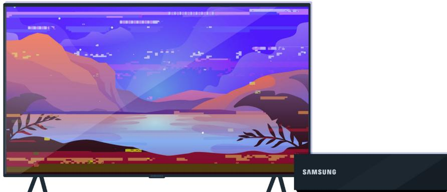
Check the antenna and input cable connections.
