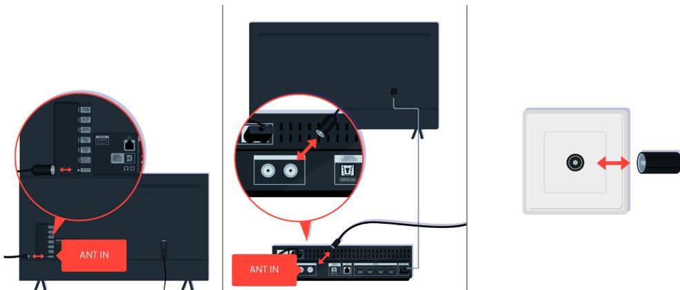
Check the antenna and input cable connections.
