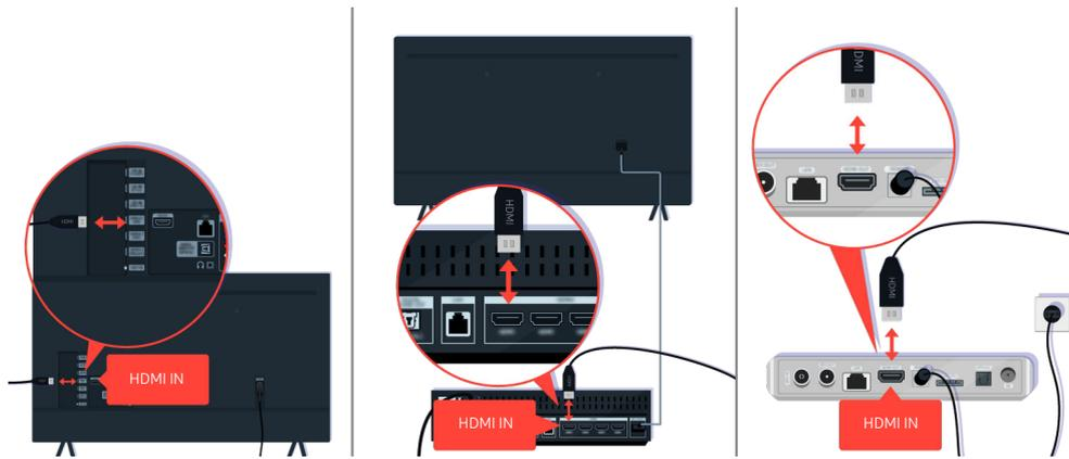
Check the antenna and HDMI cable connections.
