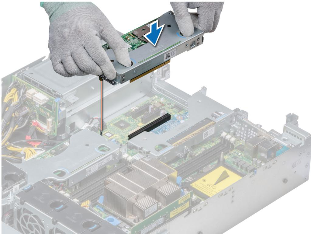
**Figure 81. Installing low profile riser left**
