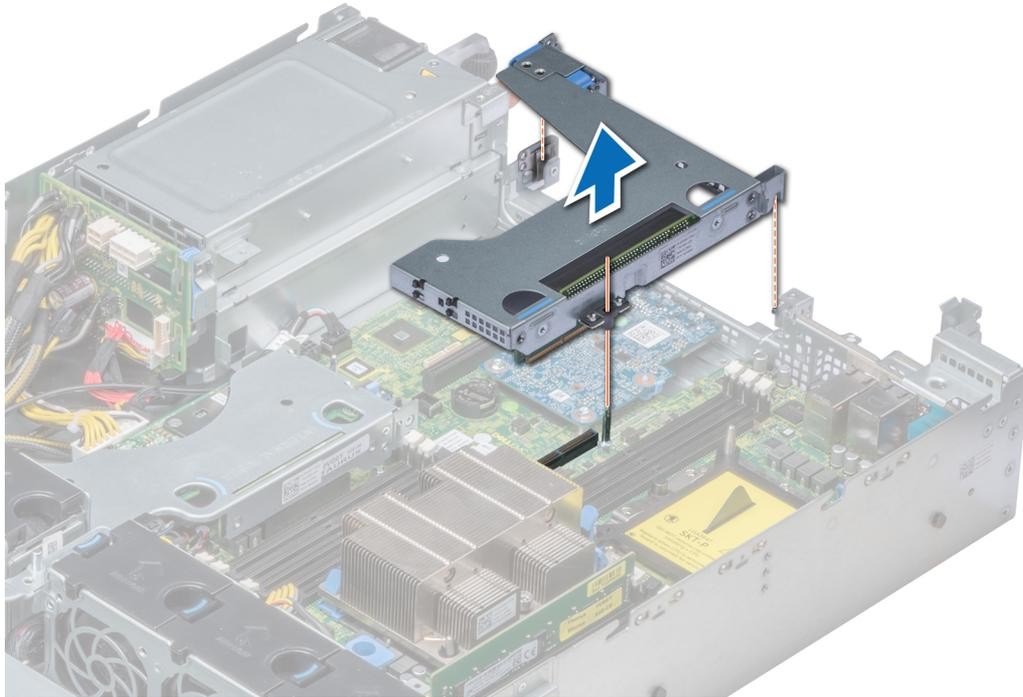
Figure 78. Removing full height X1 riser
