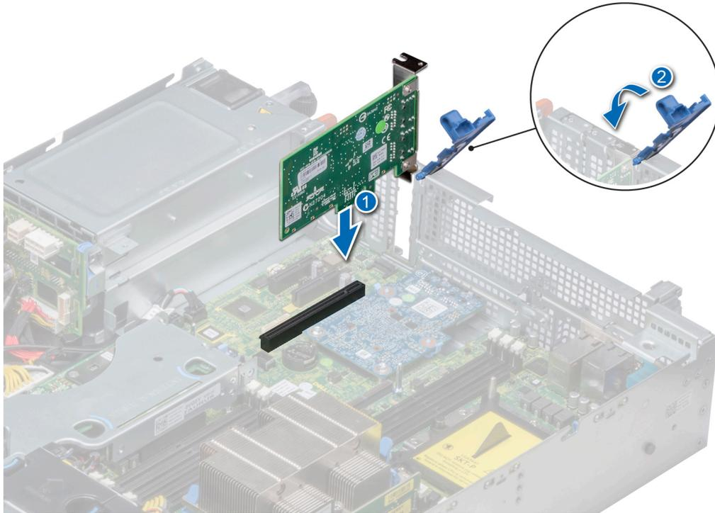
**Figure 75. Installing expansion card on system board**
