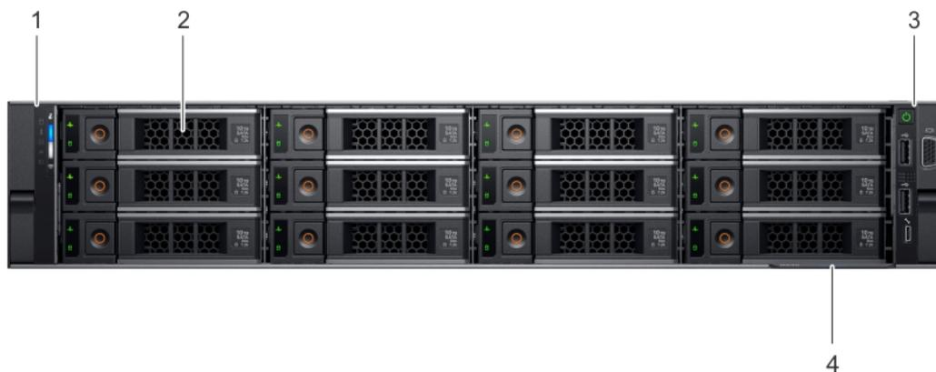
Figure 2. Front view of 12 x 3.5 inch drive system
