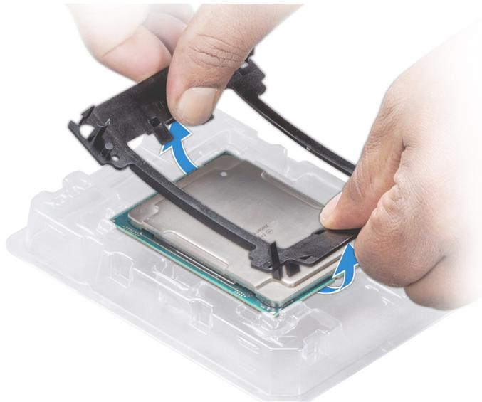
**Figure 55. Removing the processor bracket**
