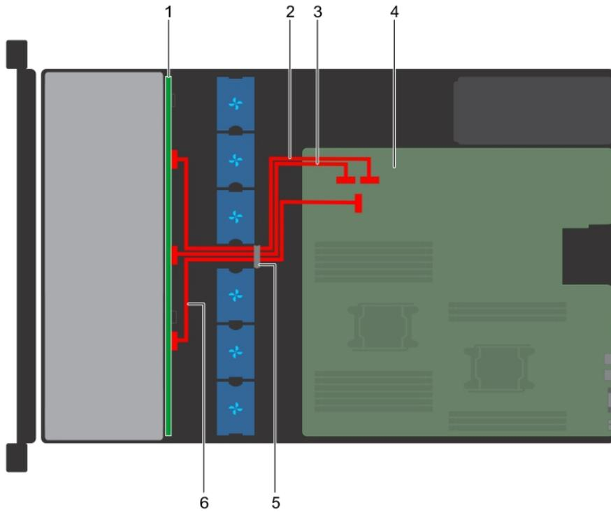
**Figure 98. Cable routing - 12 x 3.5 inch drive backplane**
