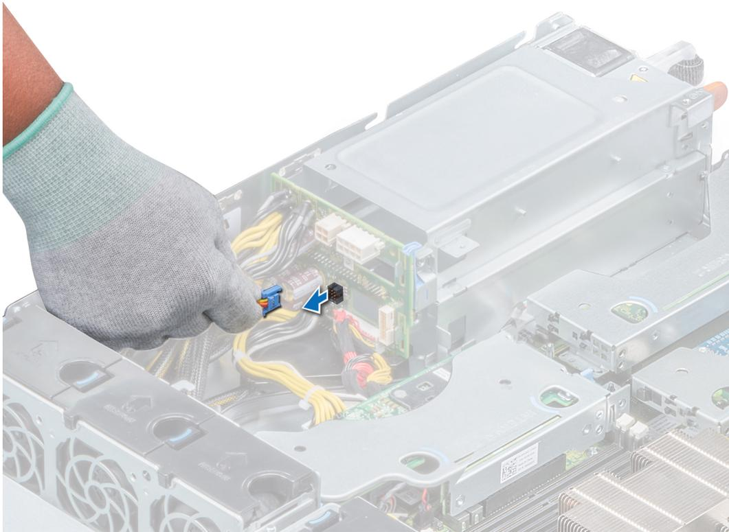
**Figure 28. Disconnecting fan cable from PIB connector**
