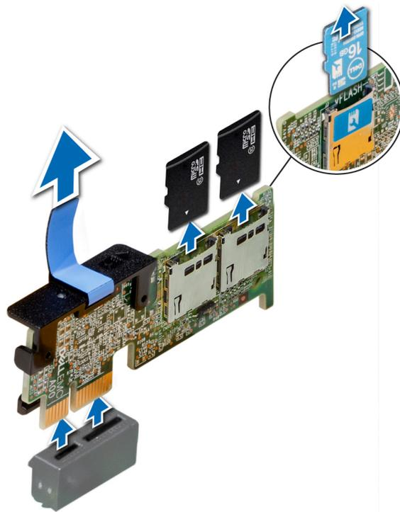
Figure 84. Removing the optional IDSDM/vFlash card
