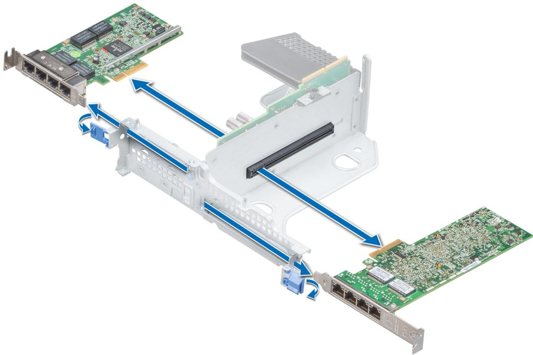
**Figure 62. Removing expansion card from butterfly riser**
