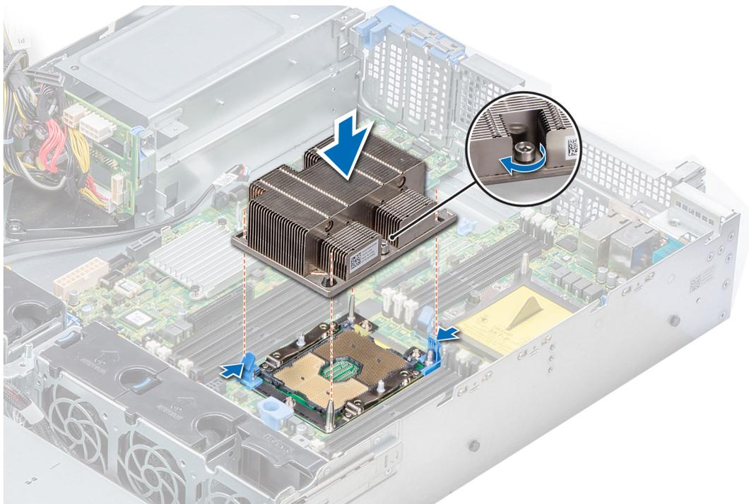
**Figure 59. Installing the processor and heat sink module**
