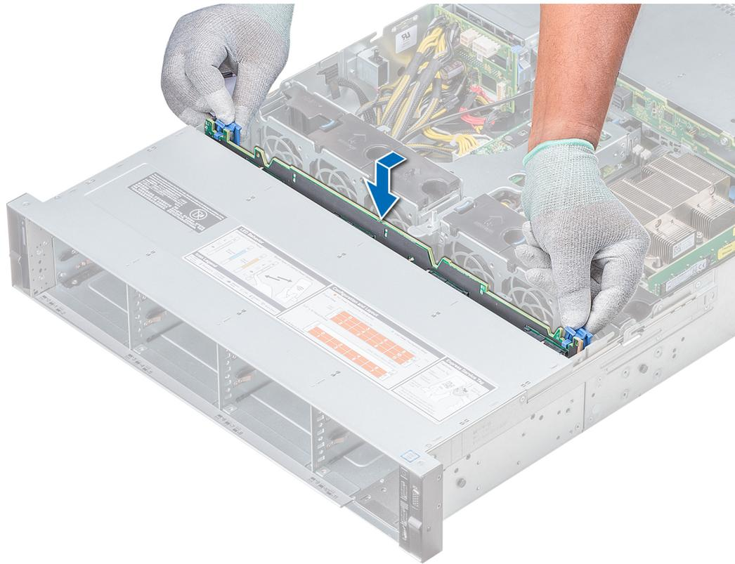
**Figure 93. Installing drive backplane**
