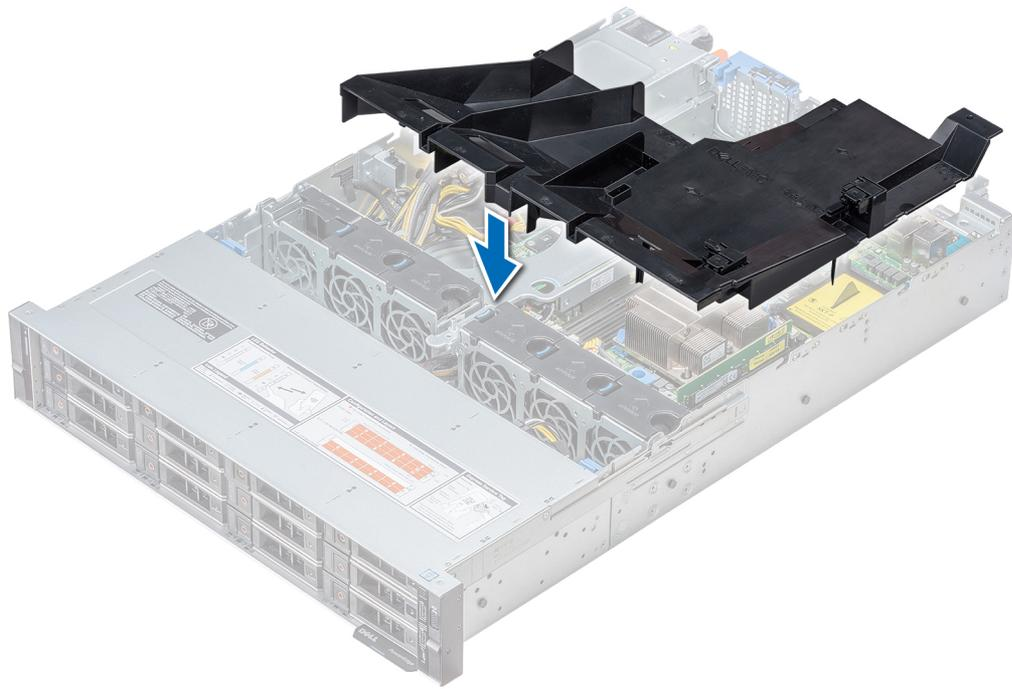
Figure 27. Installing air shroud
