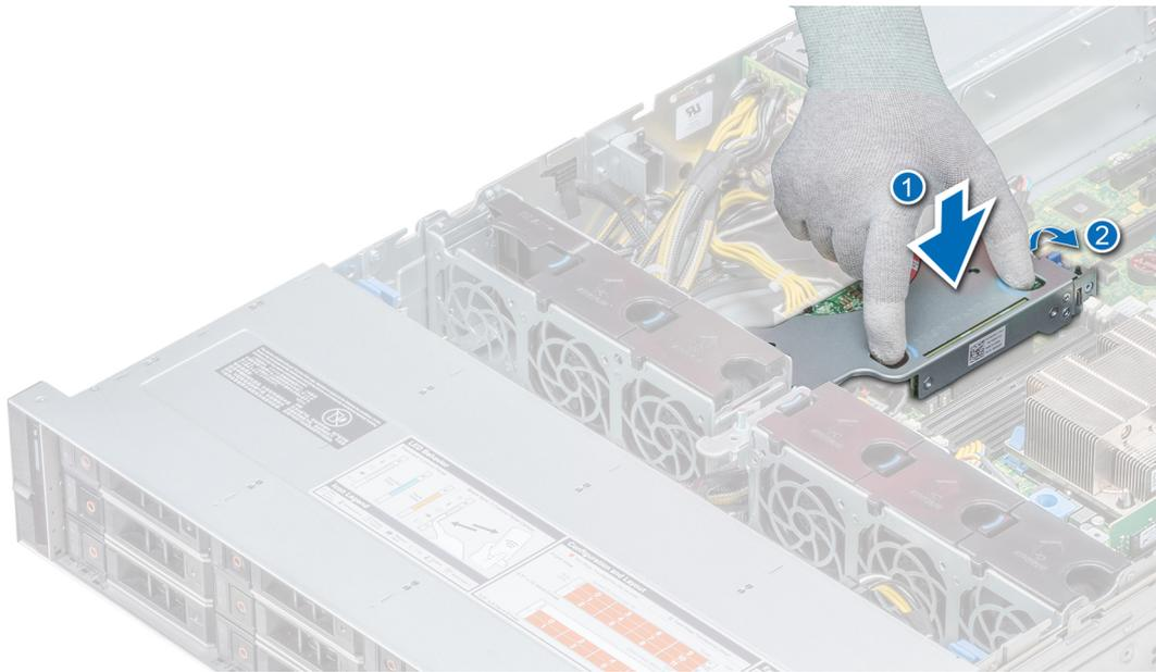
**Figure 35. Installing internal PERC riser**
