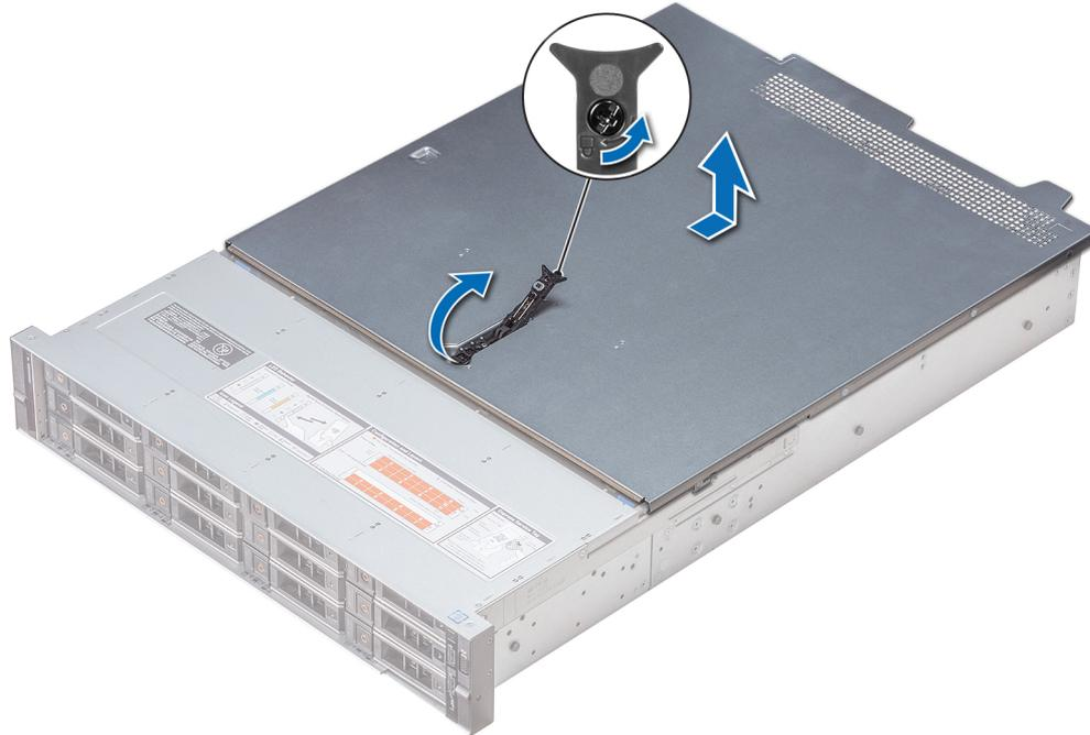
**Figure 20. Removing the system cover**
