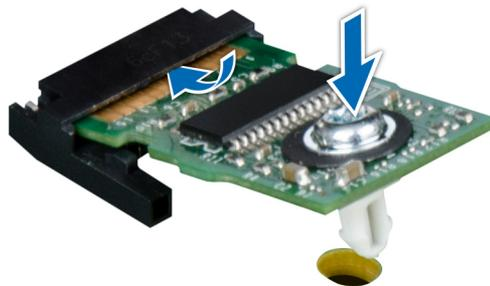
Figure 121. Installing the TPM
