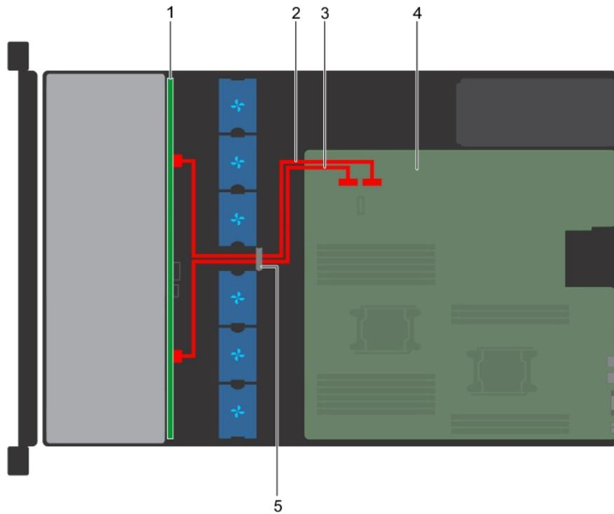
**Figure 99. Cable routing - 8 x 3.5 inch drive backplane**
