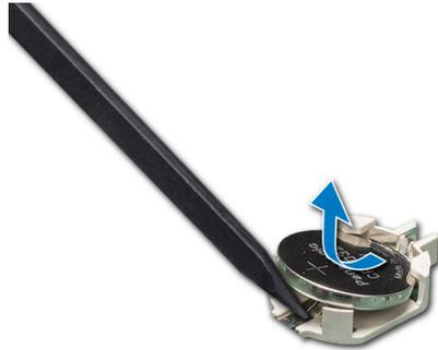
**Figure 102. Removing the system battery**
