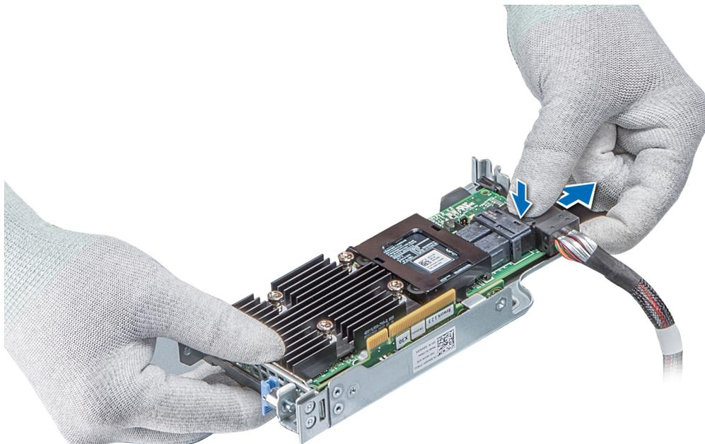
**Figure 33. Disconnecting the cable from internal PERC riser**
