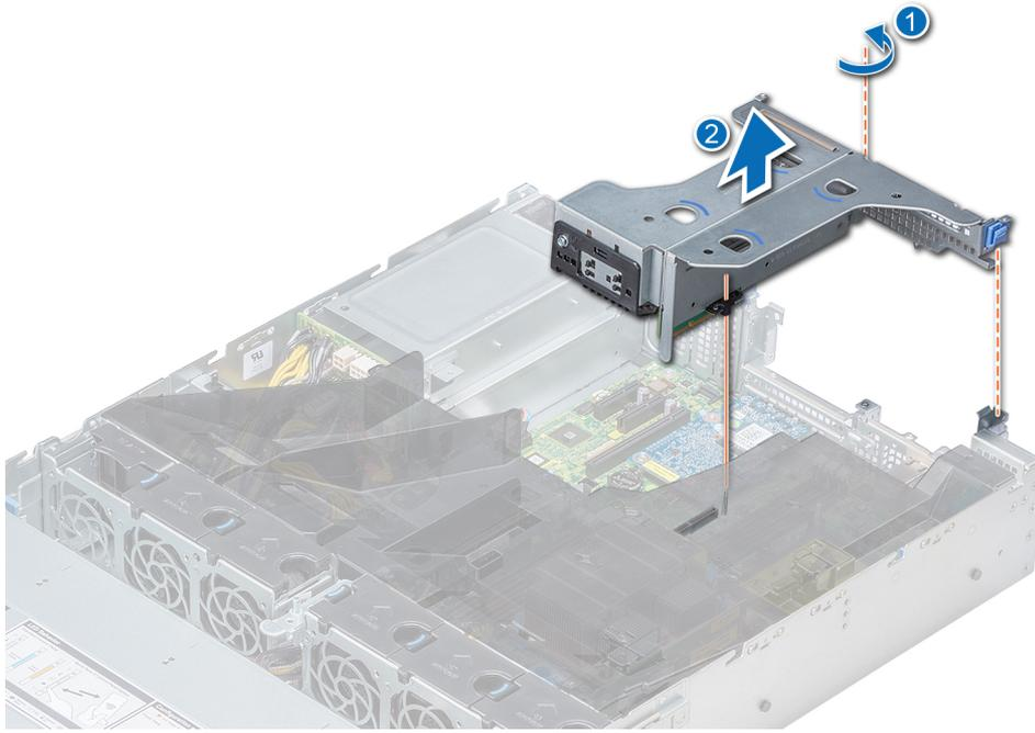
**Figure 79. Removing butterfly riser**
