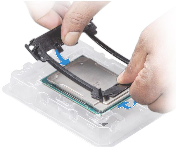
**Figure 56. Installing the processor bracket**
