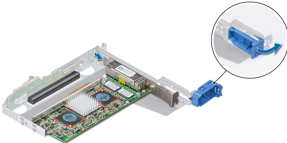
Figure 61. Removing expansion card from full height X1 riser
