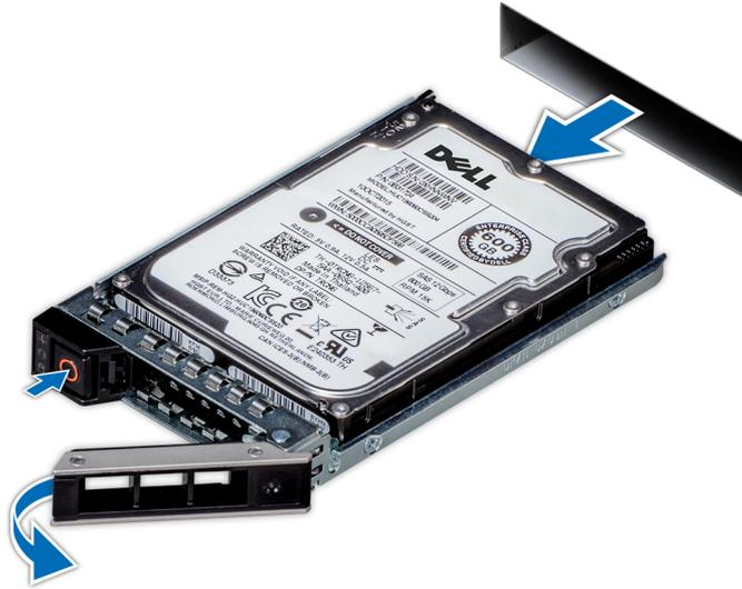
Figure 46. Removing a drive carrier
