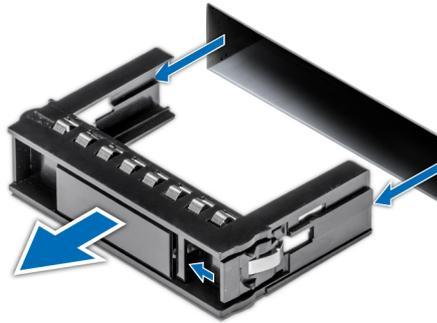
Figure 40. Removing a drive blank
