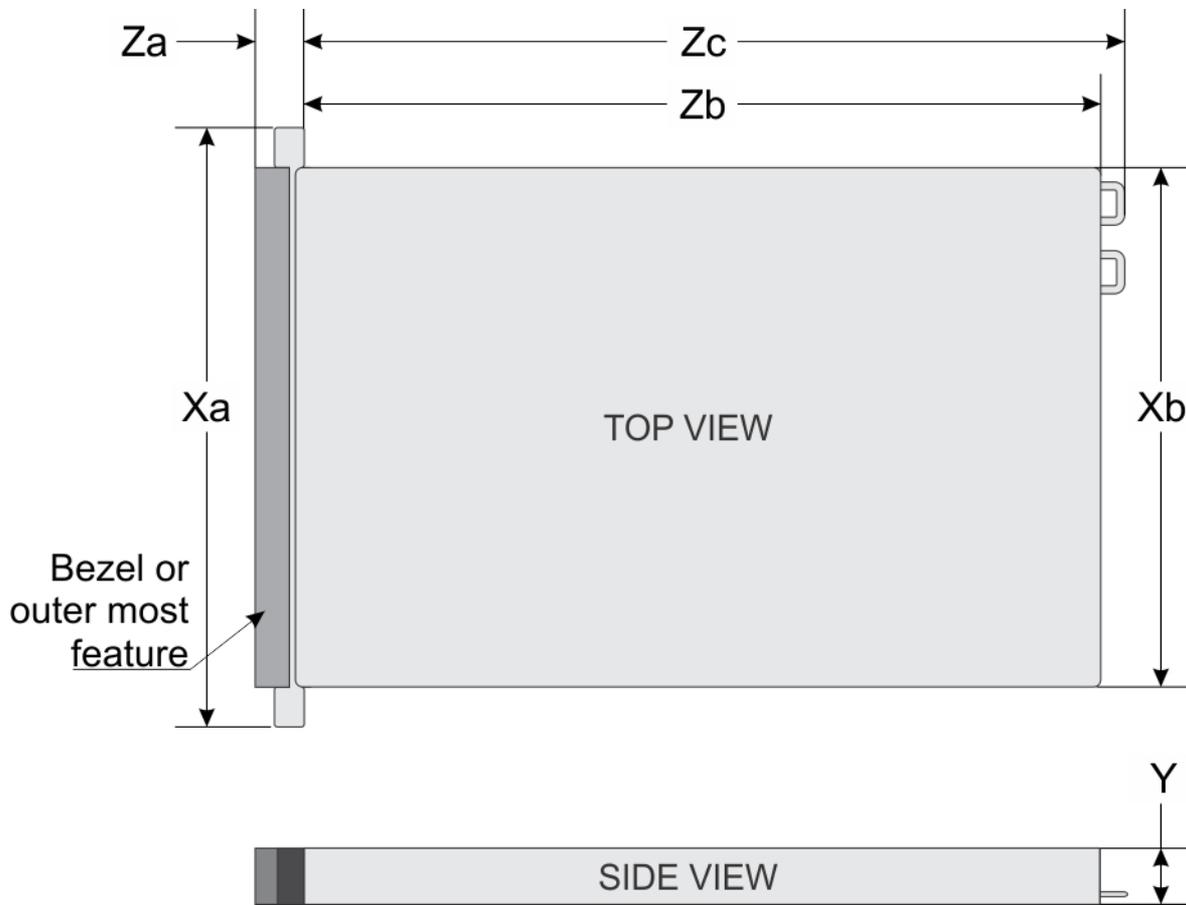
Figure 17. Dimensions of the PowerEdge R540 system
