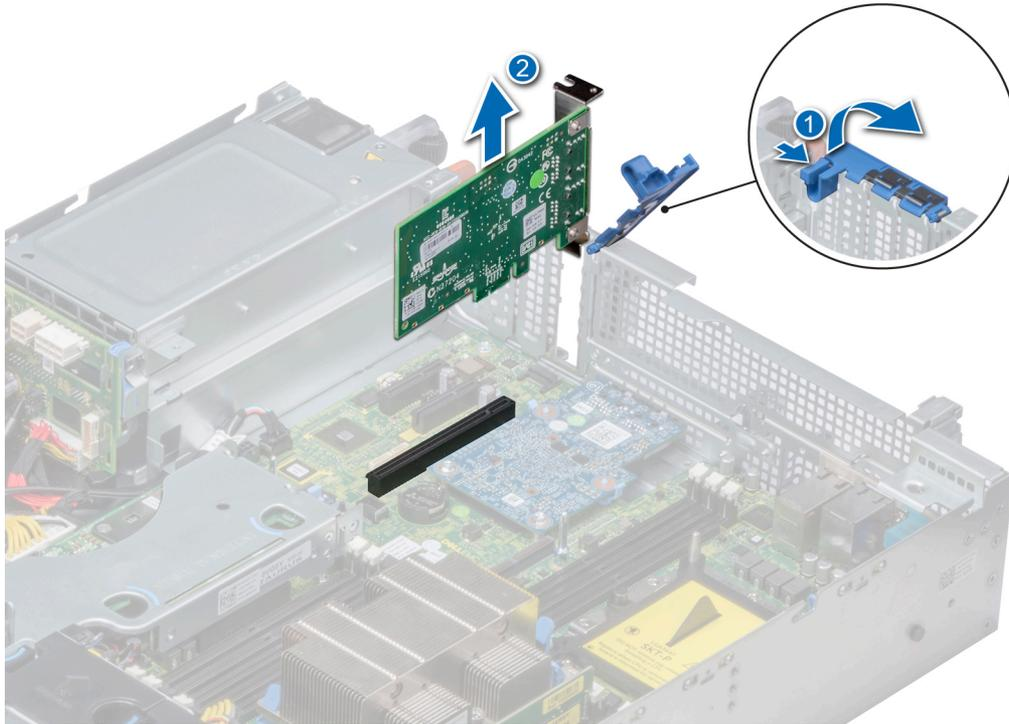
**Figure 72. Removing expansion card from system board**
