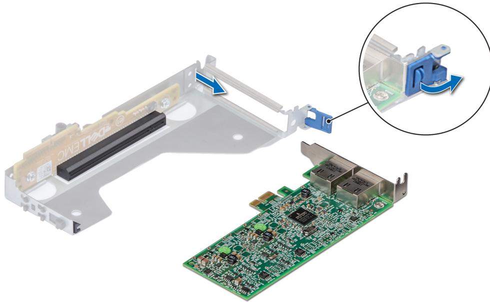
Figure 60. Removing expansion card from low profile riser
