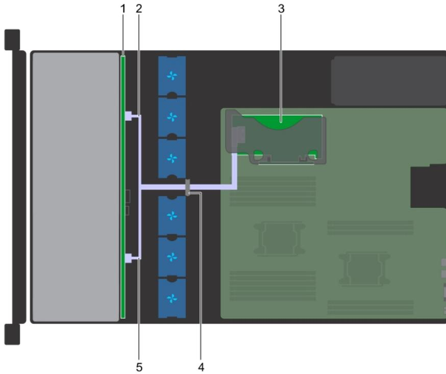
**Figure 97. Cable routing - 8 x 3.5 inch drive backplane with internal PERC riser**
