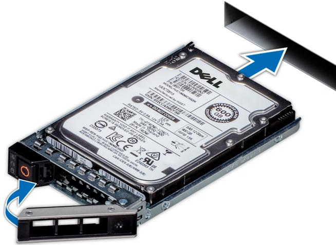
Figure 47. Installing a drive carrier
