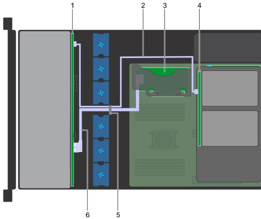
**Figure 96. Cable routing - 12 x 3.5 inch drive backplane and 2 x 3.5 inch rear drive backplane with internal PERC riser**
