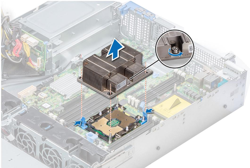
**Figure 53. Removing processor and heat sink module**
