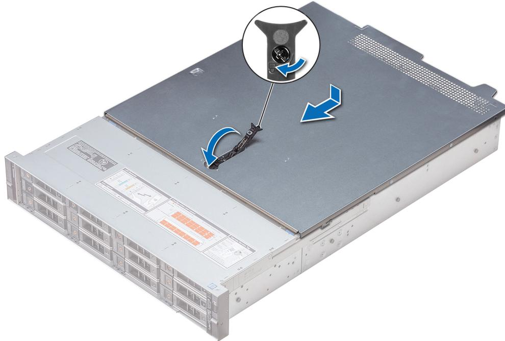
Figure 21. Installing system cover
