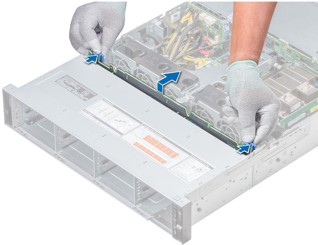
**Figure 92. Removing drive backplane**
