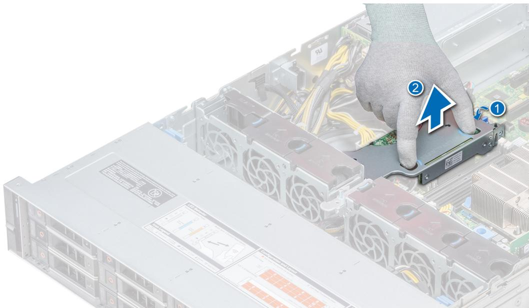
**Figure 32. Removing internal PERC riser**
