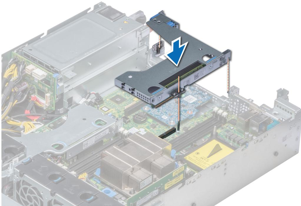
Figure 82. Installing full height X1 riser
