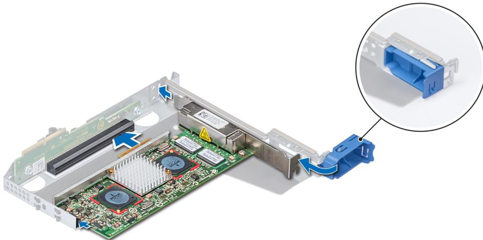
Figure 70. Installing expansion card into full height X1 riser
