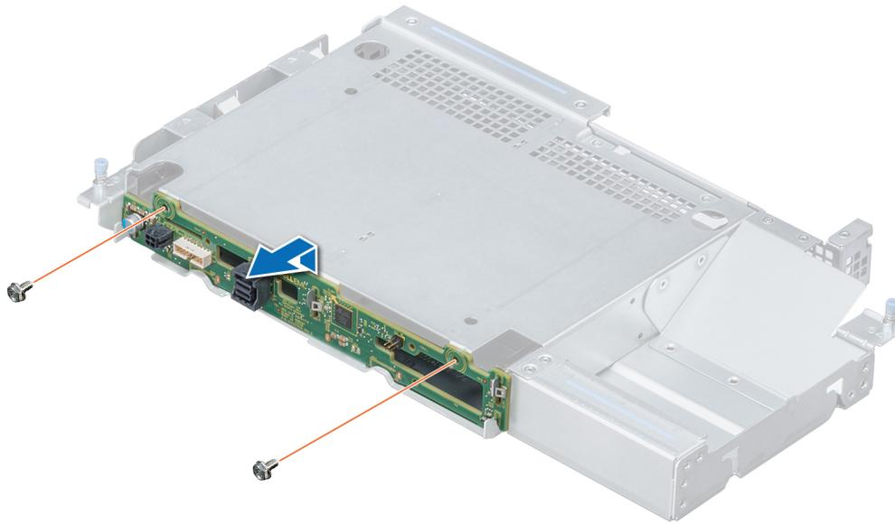
**Figure 94. Removing 3.5 inch rear drive backplane**
