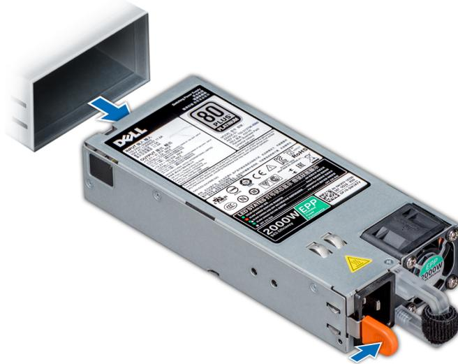
Figure 108. Removing a power supply unit
