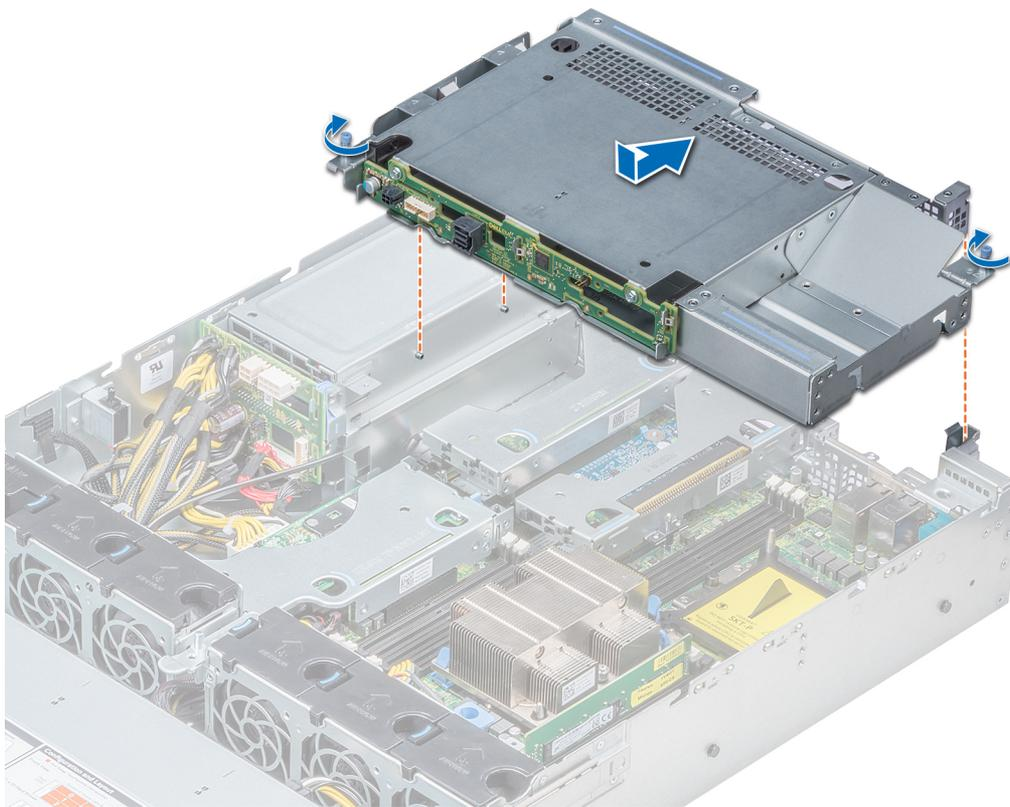
Figure 101. Installing the rear drive cage
