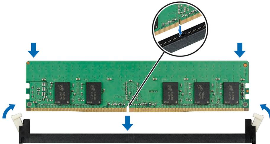
Figure 52. Installing a memory module
