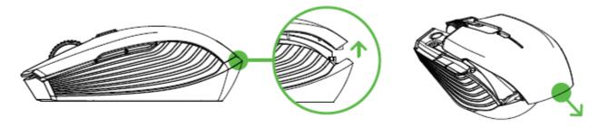
2. Insert the two included AA batteries into the Razer Atheris following the directions indicated on the battery compartment.
