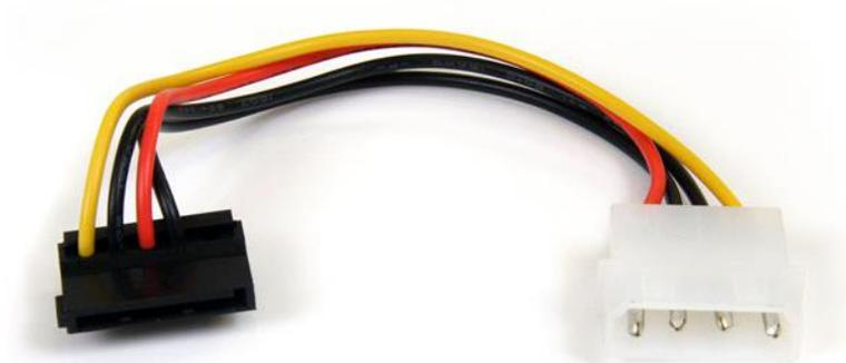
This 6-inch 4-Pin LP4 to Right Angle SATA power adapter features one 4-Pin LP4 male connector and one (female) right angle SATA power connector, allowing you to power a Serial ATA hard drive from a conventional LP4 connection, eliminating the need to upgrade the computer power supply for compatibility with the SATA hard drive.
