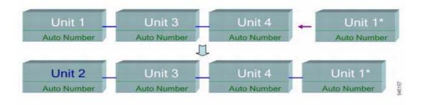
The following shows an example of auto numbering when a new unit joins the stack. The existing units retain their ID. The new unit receives the lowest available ID.
