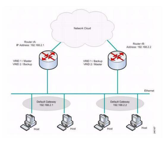
In this topology, two virtual routers are configured. For virtual router 1, rA is the owner of IP address 192.168.2.1 and is the virtual router master, and rB is the virtual router backup to rA. Clients 1 and 2 are configured with the default gateway IP address of 192.168.2.1.
