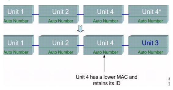
NOTE If a new stack has more than the maximum number of units (8), all extra units are shut down.
