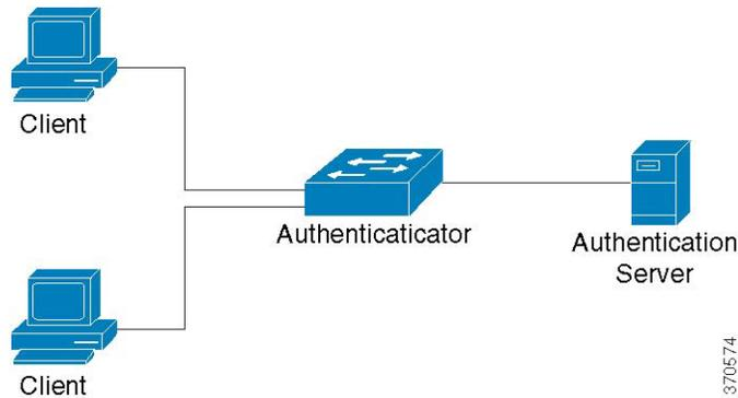
A network device can be either a client/supplicant, authenticator or both per port.
