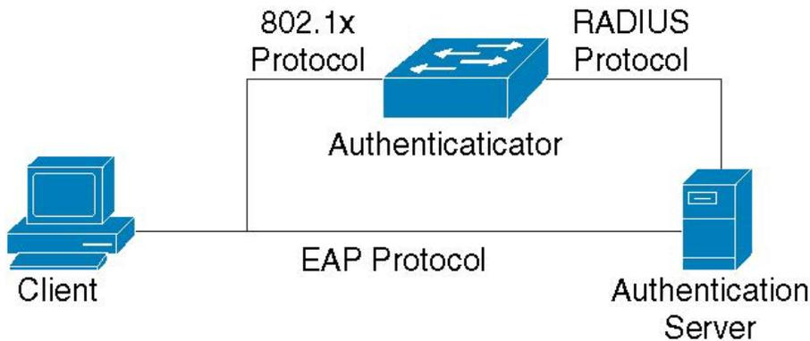
The device supports the 802.1x authentication mechanism, as described in the standard, to authenticate and authorize 802.1x supplicants.
