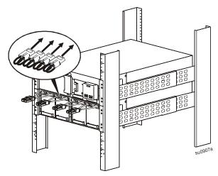
**UPS models SRT5K or SRT6K with one XLBP** Install one XLBP bezel and one UPS bezel.
