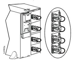
**2** Reinstall the battery compartment doors. Tighten the thumbscrews to secure two doors.
