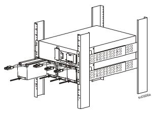
Reinstall the battery compartment doors.
