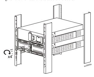
**UPS models SRT8K or SRT10K with one XLBP** Install one XLBP bezel and two UPS bezels.
