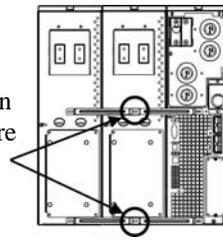
4. Connect the green/yellow ground wires (screws included), as shown in the diagrams below.
