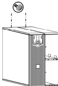
*Installing and Connecting the Front Batteries and Attaching the Bezel*
