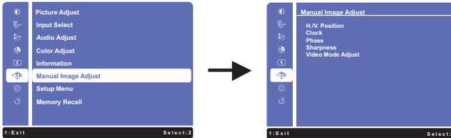
An adjustment page appears after you press the **2** Button. Then, select V. Position by using the **▲ / ▼** Buttons. Press the **2** Button again. Then, use the **▲ / ▼** Buttons to change the vertical position settings. The vertical position of the overall display should be changing accordingly while you are doing this.
