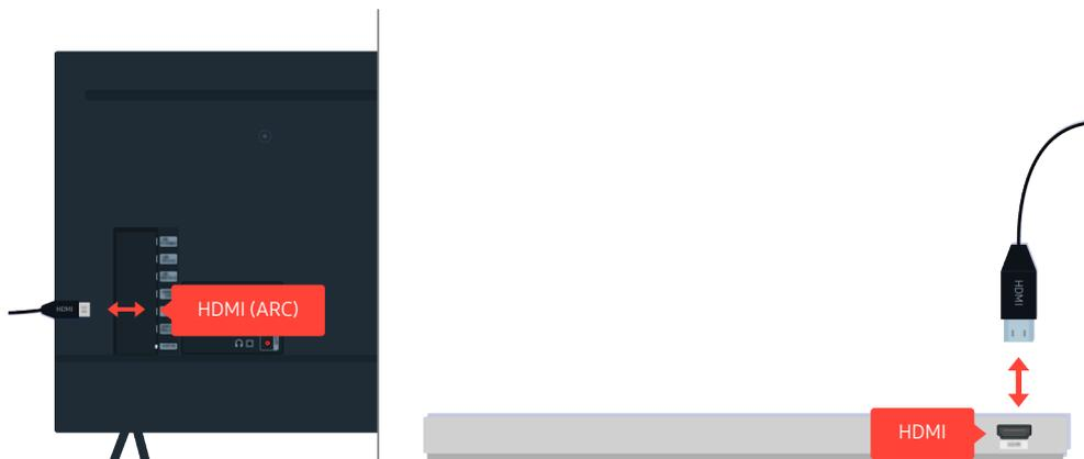
If no sound comes out of your Sound Bar and if it is connected to the TV with an HDMI cable, check the HDMI (ARC) connector on the back of the TV.
