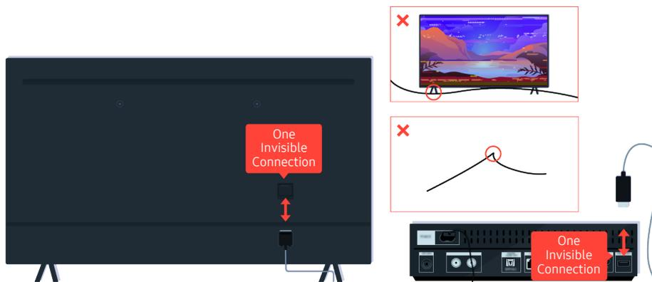
If the problem persists and if your TV uses the One Invisible Connection, disconnect and reconnect the One Invisible Connection to the TV and the One Connect (OC) Box. Ensure that the One Invisible Connection is not pinched or bent sharply.
