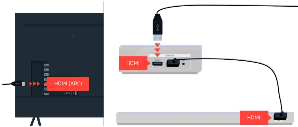
If your Sound Bar is connected to a receiver, and the receiver is connected to the TV using an HDMI cable, check the HDMI connector on the back of the TV. The cable must be connected to the HDMI (ARC) port on your TV.
