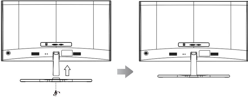
Remove: Press release bottom and reverse the steps to remove the base.
