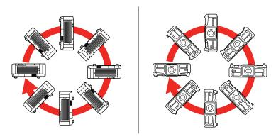
If you project from the ceiling or from the rear, select the correct **Projection** setting and, if necessary, turn on the **Inv Direction Button** setting and adjust the **OSD Rotation** setting.
