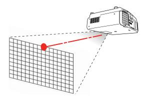
**Note:** If you installed the optional ELPLU02 short throw lens and you see a message prompting you to manually adjust the image distortion, manually rotate the distortion ring counterclockwise. Adjust the focus and then rotate the distortion ring to correct image distortion.
