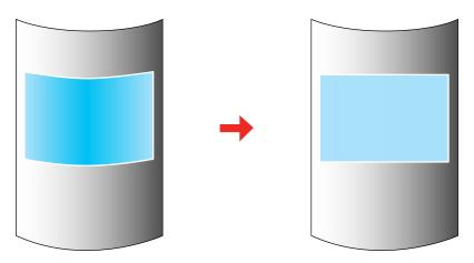
**Note:** For the best results, project from the front of the screen onto a surface with a uniform arc radius and with the lens in the home position. The image may not be evenly focused throughout even after performing the steps here. If you see a 4K Enhancement message, select **Yes** to disable the 4K Enhancement feature.
