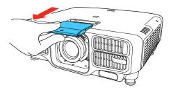
4. Hold the lens firmly as you slide the lock lever to the **Release** position (as shown) until you hear it click.
