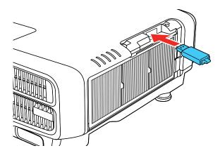
**Note:** Connect the flash drive directly to the projector. Do not use a hub or your settings may not be saved correctly.
