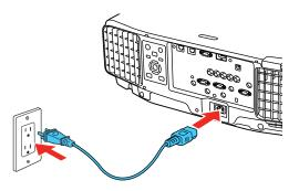
2. Plug the power cord into an electrical outlet.
