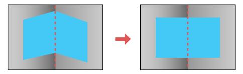
**Note:** For the best results, project from the front of the screen onto a right-angled surface and with the lens in the home position. The image may not be evenly focused throughout even after performing the steps here. If you see a 4K Enhancement message, select **Yes** to disable the 4K Enhancement feature. Corner Wall is not supported for the ELPLX01 lens.
