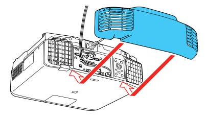
3. Tighten both cable cover screws.
