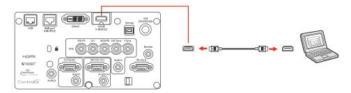
**Note:** The projector converts the digital audio signal sent from your computer into a mono analog signal for the internal speaker or a stereo analog signal if you are connecting to external speakers.
