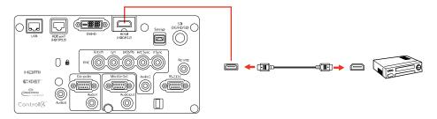
**Note:** The projector converts the digital audio signal sent from your video source into a mono analog signal for the internal speaker or a stereo analog signal if you are connecting to external speakers.
