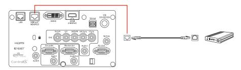
**Note:** See the documentation that came with the HDBaseT transmitter for instructions on connecting it to your video device or computer.
