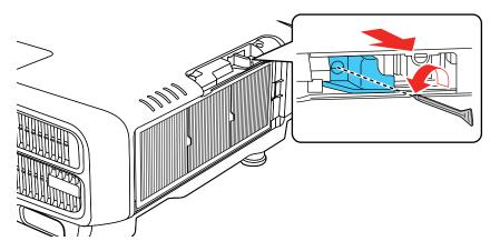
4. Insert the wireless LAN module into the port.
