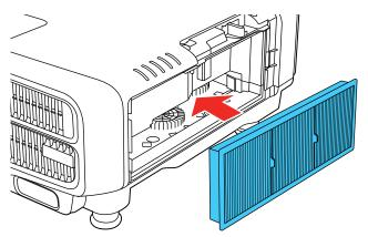
7. Attach the air filter cover as shown, and press it gently until it clicks into place.
