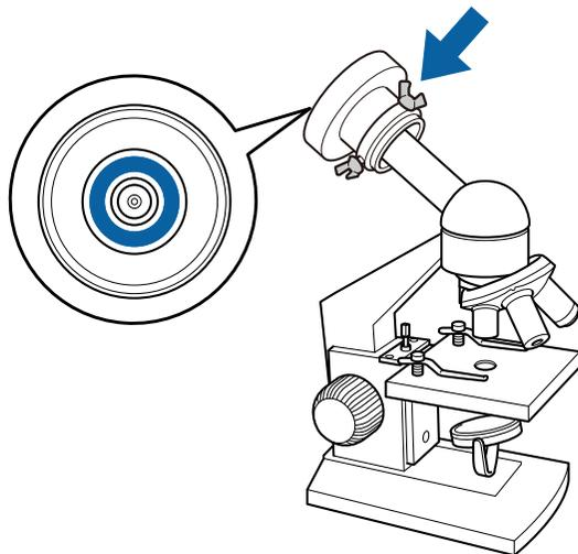
**3** Adjust the height and angle of the camera head, and then attach it to the microscope adapter.
