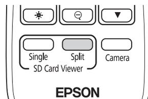
A live image and an image on the SD card are displayed side-by-side on the screen.
