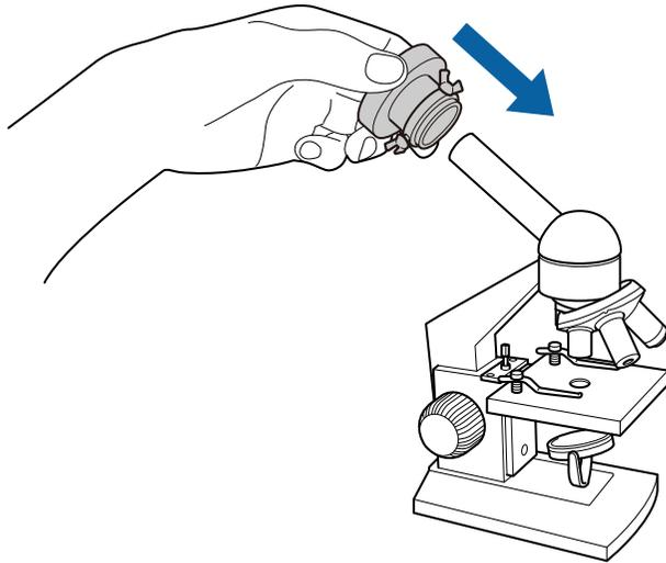
**2** With the microscope's eye piece in the center of the microscope adapter, tighten the three screws on the microscope adapter to secure it in place.
