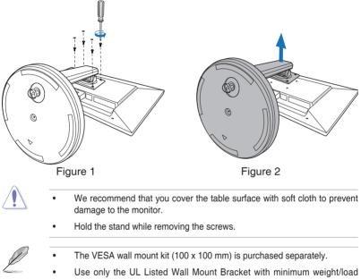
Use only the UL Listed Wall Mount Bracket with minimum weight/load 22.7kg (Screw size: M4 x 10 mm)
