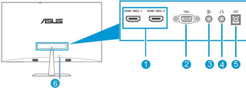
1. **HDMI/MHL port:** This port is for connection with an HDMI/MHL compatible device.
