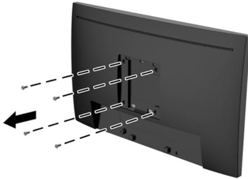
3. Install the mounting plate to the wall or swing arm of your choice using the four screws that were removed from the VESA holes on the rear of the display head.
