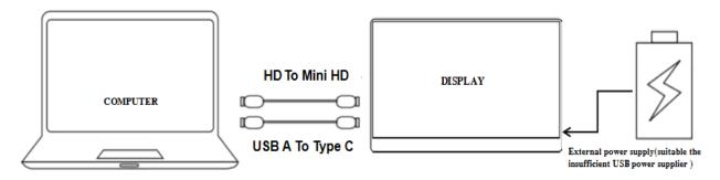
When connecting to a compatible computer using the HDMI interface, you need to connect the supplied HDMI cable between the computer and the display. You should also connect the display to the computer via USB, using a USB to USB Type C cable (Not supplied), connected to the left-hand Main USB Type C socket on the left of the display.
