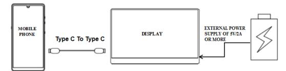
When there is no external power supply connected to the secondary USB Type C socket on the right of the display, the mobile phone battery will supply power to the display. To reduce power usage the energy-saving mode will be activated and the display brightness will be reduced to 30%, and the user can adjust the brightness and volume of the display according to the output power of the mobile phone).
