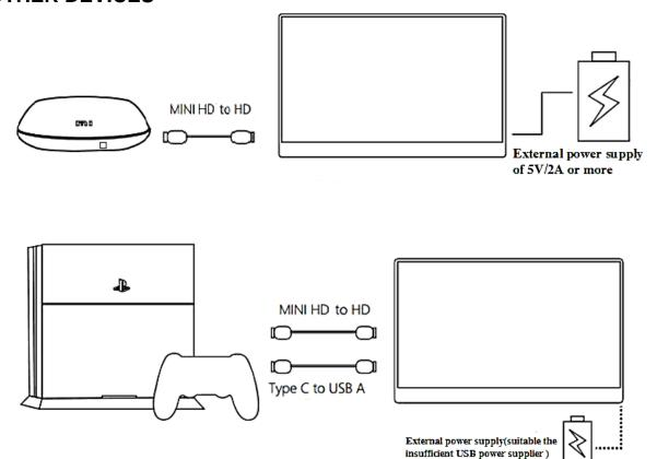
When connecting a device using HDMI, be sure to connect the power cable first, then connect the HDMI to ensure the smooth transmission of the signal.
