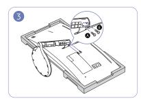
Rotate A and B screws for fixing.
