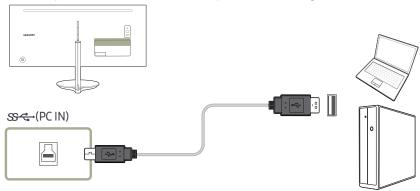
Connect the USB cable to an the back of the product and USB on the PC.
