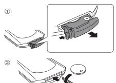
• Set the button-type battery with its (+) mark facing upward.
