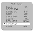
2. Select a desired mode using the Function Setup switch.
