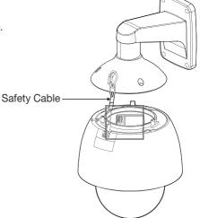
**4.** Assemble Camera and Installation Base Assemble the installation base and camera by matching the installation direction guides.
