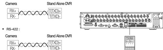
Connecting with the Samsung Techwin Controller SPC-6000
