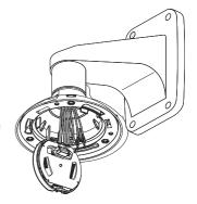
3. Connect the camera safety wire to the installation base.
