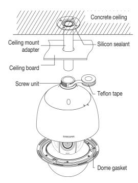
Take particular caution to ensure that there is proper sealing if the installed side is not flat.
