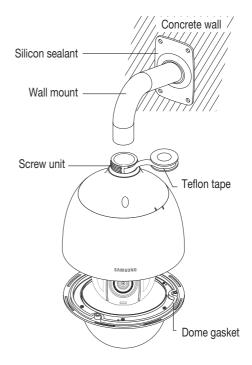
Take particular caution to ensure that there is proper sealing if the installed side is not flat.
