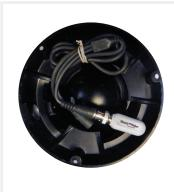
Install a Balun within the base of the camera.
